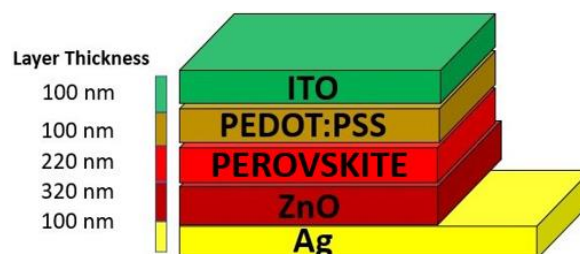
Fig. 16. Simulated Perovskite Solar cell with layer Thickness
