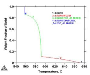
**Fig.2.** The solid fraction-temperature diagram achieved by Thermocalc.
