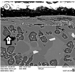
Fig.13. The subsurface area of the Specimens worn at the applied loads of (a) 25N and (b) 75N. Cracks in particle shown by arrow numbered 1. Formation of tribolayer (MML) during the wear process can be apparently seen.
