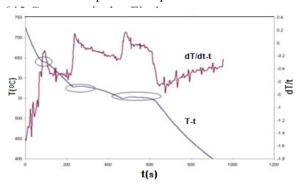
**Fig.1.** The cooling curve of the composite and its corresponding differentiated curve.
