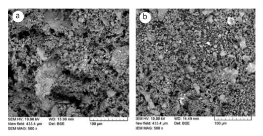
**Fig.11.** Debris particles collected from the specimen worn at the applied load of 75N (a) As-cast. (b) After thixoforming with 10% reduction of area.
