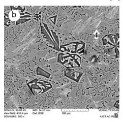
Fig.3. (a) Typical microstructure of the Al-20wt%Mg<sub>2</sub>Si composite, as-cast at 700°C. (b) The same as (a) at higher magnification. 1-Primary Mg<sub>2</sub>Si, 2-Binary <sub>Eu</sub>, 3-Si<sub>Eu</sub>, 4-Iron-rich intermetallic
