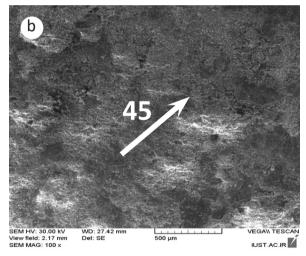
Fig.7. The worn surface of the Al-20%wtMg<sub>2</sub>Si alloy at the applied load of 25 N (a) as-cast (b) thixo-formed.
