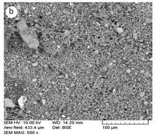
**Fig.8.** Wear debris collected from the specimens worn at the applied load of 25N (a) as-cast (b) thixo-formed with 10% reduction of area.
