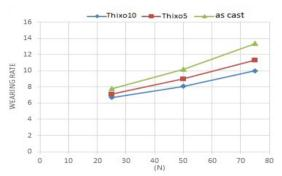
Fig. 6. Wear rate variations versus the applied load.
