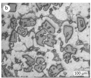
Fig. 4. The composite microstructure heated at 575 °C for 45 minutes with (a) 10% reduction of area (b) 5% reduction of area
