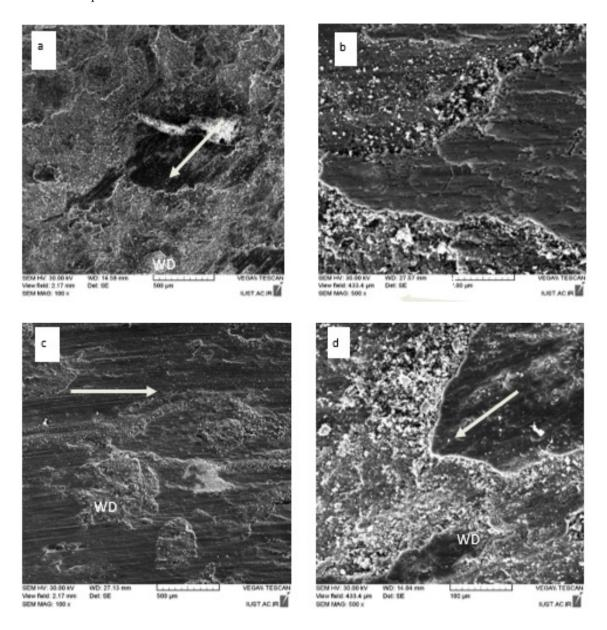
Fig.10. The plan view of the worn surfaces of the Al-Mg, Si alloy worn at the applied load of 75 N: (a) As-cast. (b) Higher magnification of (a). (c) After thixoforming with 10% reduction of area. (d) Higher magnification of (c).
