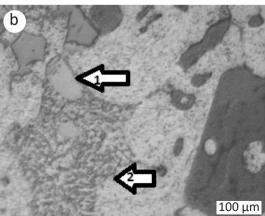
Fig.5. Distribution of α-Al and Mg<sub>2</sub>Si particles in the composite heated at 575 °C for 45 minutes with 10% reduction of area (b) The same as (a) but at higher magnification. 1-Iron-rich intermetallic. 2- Si Eutectic.
